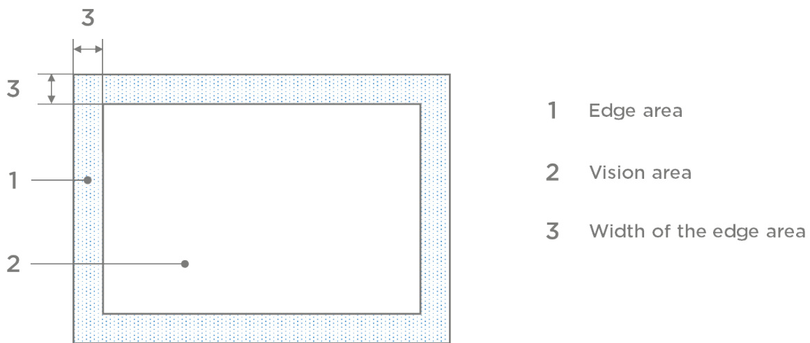
Picture 25: Edge and vision area for laminated glasses according to ÖNORM EN 12543-6
